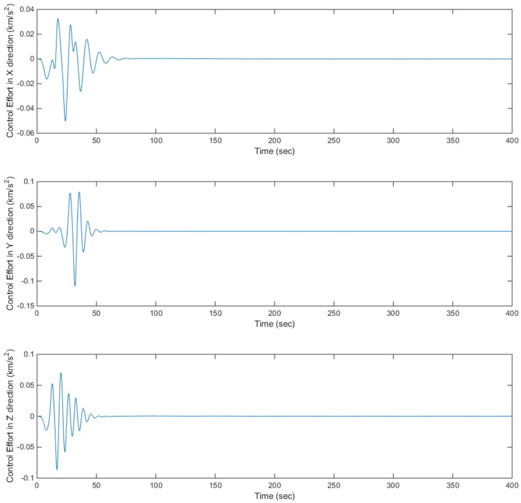
**Fig. 8** Control Effort required while using Optimal Trajectory Tracking for Docking
