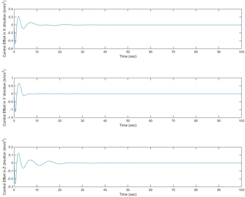
**Fig. 5 Control Effort required while using Direct Adaptive Controller for Docking**
