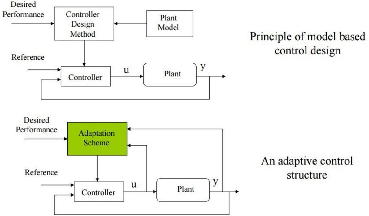
**Fig. 1 Structure of an Adaptive System (Landau, Lonzano, M'Saad, and Karimi. 2011)**
