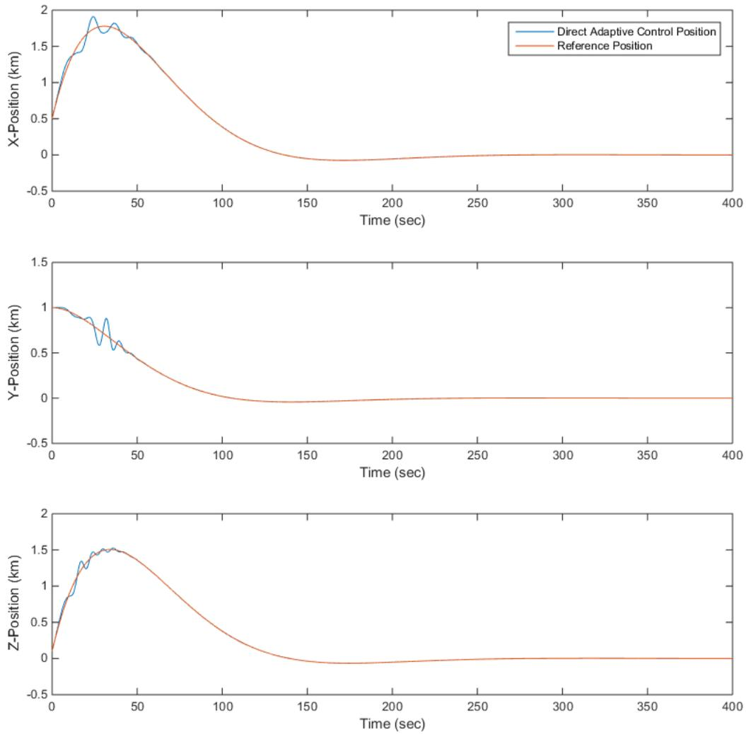
**Fig. 6 Relative Position w.r.t Chief while using Optimal Trajectory Tracking for Docking** disturbances. This is evident from the magnitude of disturbance, which is around  $10^{-7}$ . This can be observed in the figure 9 below:
