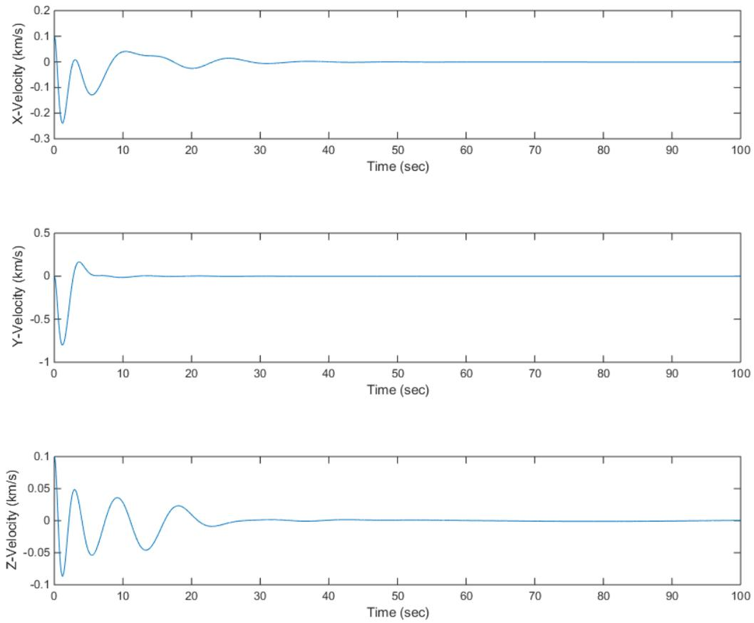
**Fig. 4 Relative Velocity w.r.t Chief while using Direct Adaptive Controller for Docking**
