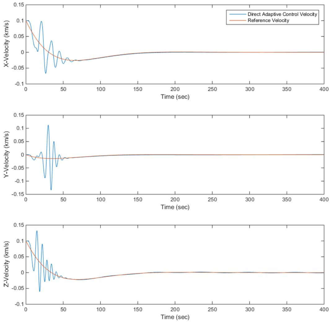
**Fig. 7 Relative Velocity w.r.t Chief while using Optimal Trajectory Tracking for Docking**
