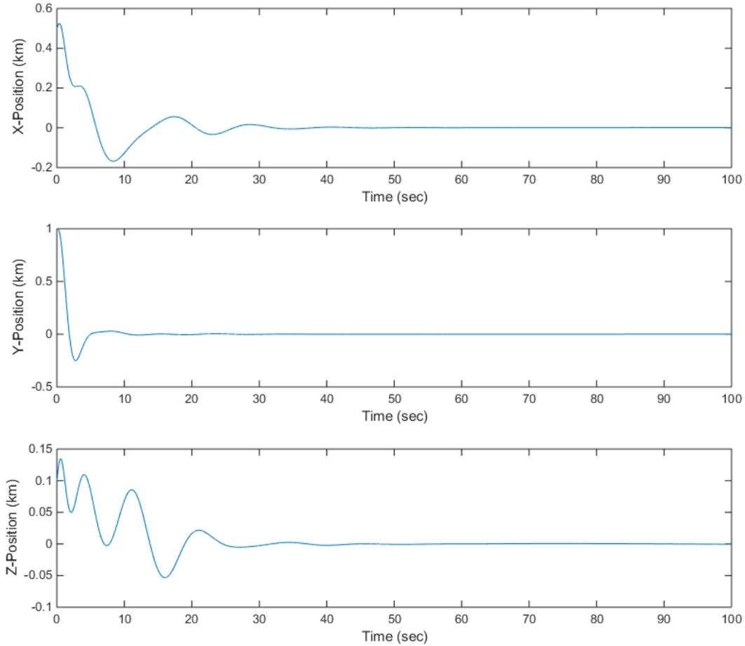
**Fig. 3 Relative Position w.r.t Chief while using Direct Adaptive Controller for Docking**
