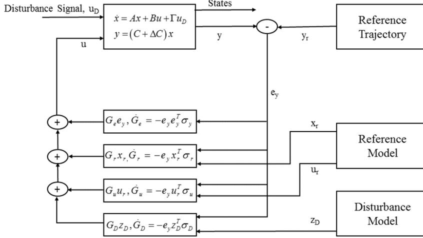
**Fig. 2 Adaptive Control System Architecture**
